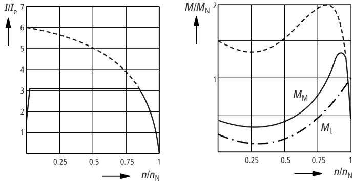
Motors with a low pull-up torque may not be able to develop enough torque during soft start operation. As a result, the drive will not start as required, and will remain at a certain speed, whereas it would start-up as required if it was connected directly to the mains.
