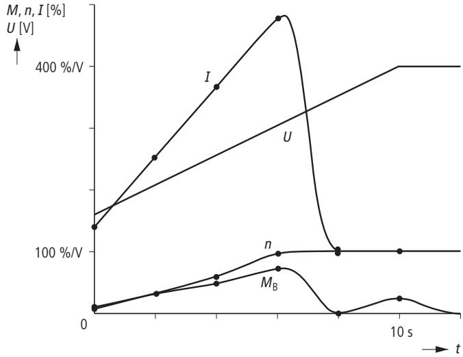
With a suitable calculation program, the following graph was calculated for the same drive. In this case, the ramp was divided into 250 increments (For comparison: our example had 5 increments).
