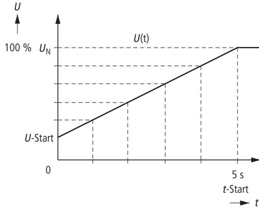
The motor is stationary for the first step. The soft starter outputs a voltage of 20 % of the mains voltage. The motor used in the example has the following data:
